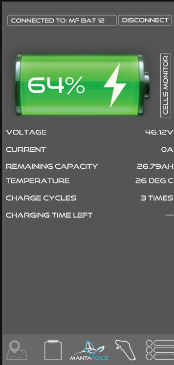
Once battery is connected, the battery charge percent is visible along with other battery parameters. Swipe right to monitor battery cells
