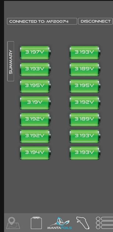
The battery cells are displayed on this page. the cumulative value is the present total voltage of the battery.
