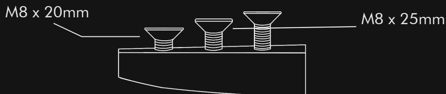
Use allen key from the provided tool kit and tighten the wing to the efoil. The wing must not wobble on the efoil and must sit sturdy in place.
